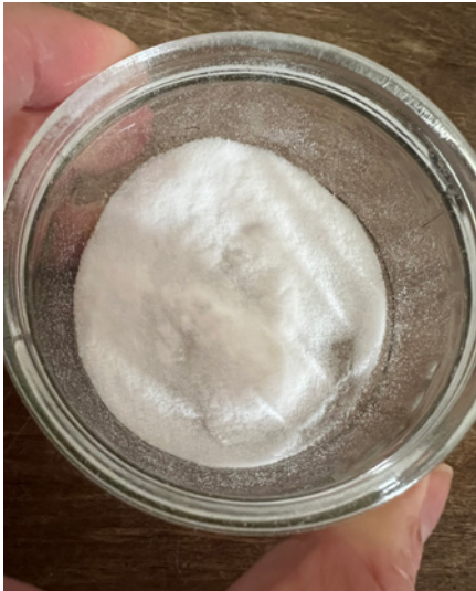
Figure 3. Hollow glass microspheres (© Dr R Ellis)
